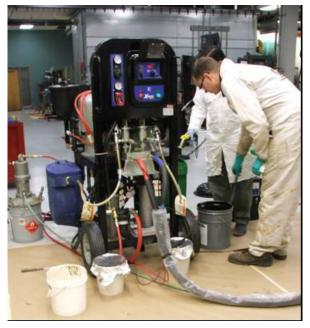
FIGURE A-3. Plural component reaction spray equipment.
