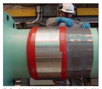
FIGURE A-12. Completion of shaft-to-sleeve fairing with sealing/fairing compound.
