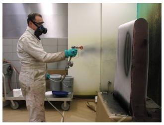
FIGURE A-7. Reaction spray of elastomeric coating.
