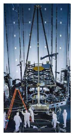
Inside a vacuum chamber at NASA's Johnson Space Center in Houston, the James Webb Space Telescope's Pathfinder backplane test model is being prepared for its cryogenic test. (NASA photo)
