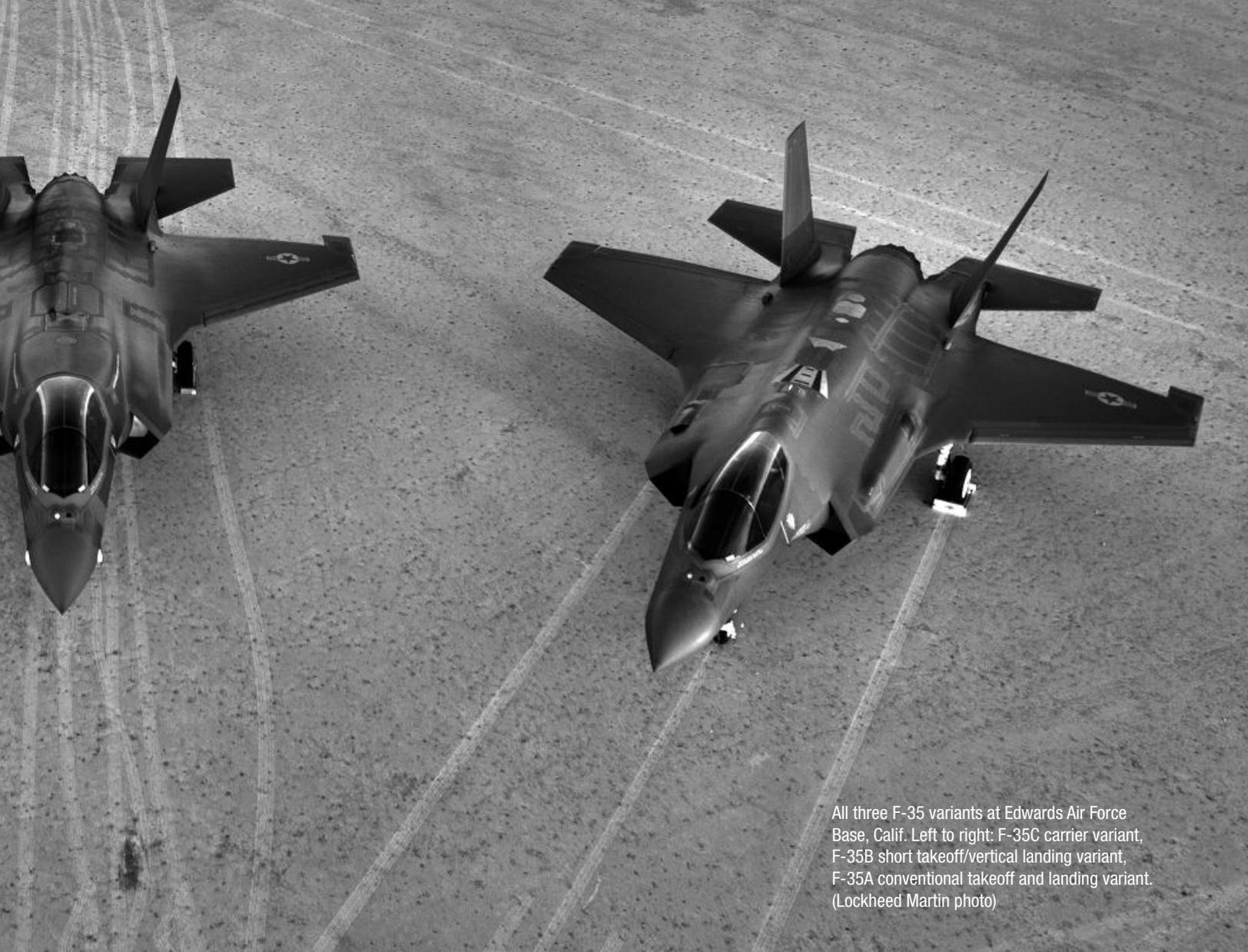
All three F-35 variants at Edwards Air Force Base, Calif. Left to right: F-35C carrier variant, F-35B short takeoff/vertical landing variant, F-35A conventional takeoff and landing variant. (Lockheed Martin photo)
