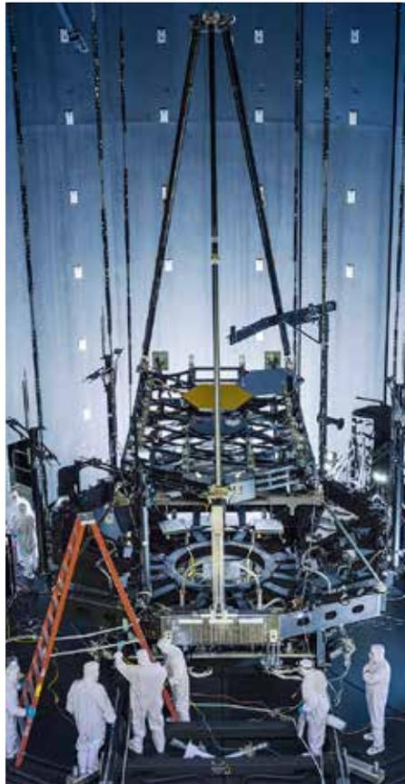
Inside a vacuum chamber at NASA's Johnson Space Center in Houston, the James Webb Space Telescope's Pathfinder backplane test model is being prepared for its cryogenic test. (NASA photo)
