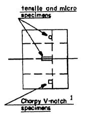
NOTE: The symbols used indicate the location of specimens on this diagram and are not required marking for the specimens (see 3.18.1).
