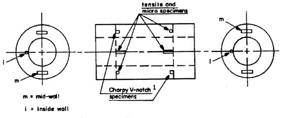
1. See 4.4.3.2.7 for specific location of Charpy V-notch specimens. NOTE: The symbols used indicate the location of specimens on this diagram and are not required marking for specimens (see 3,18,1).
