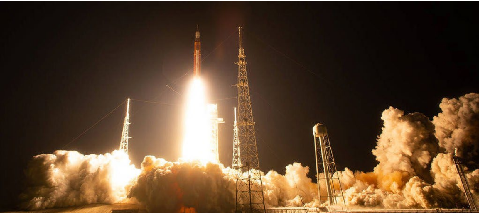
NASA's Space Launch System rocket carrying the Orion spacecraft launches on the Artemis I flight test, Wednesday, Nov. 16, 2022, from Launch Complex 39B at NASA's Kennedy Space Center in Florida. NASA's Artemis I mission is the first integrated flight test of the agency's deep space exploration systems: the Orion spacecraft, Space Launch System (SLS) rocket, and ground systems. SLS and Orion launched at 1:47 a.m. EST, from Launch Pad 39B at the Kennedy Space Center. Photo Credit: (NASA/Joel Kowsky)
