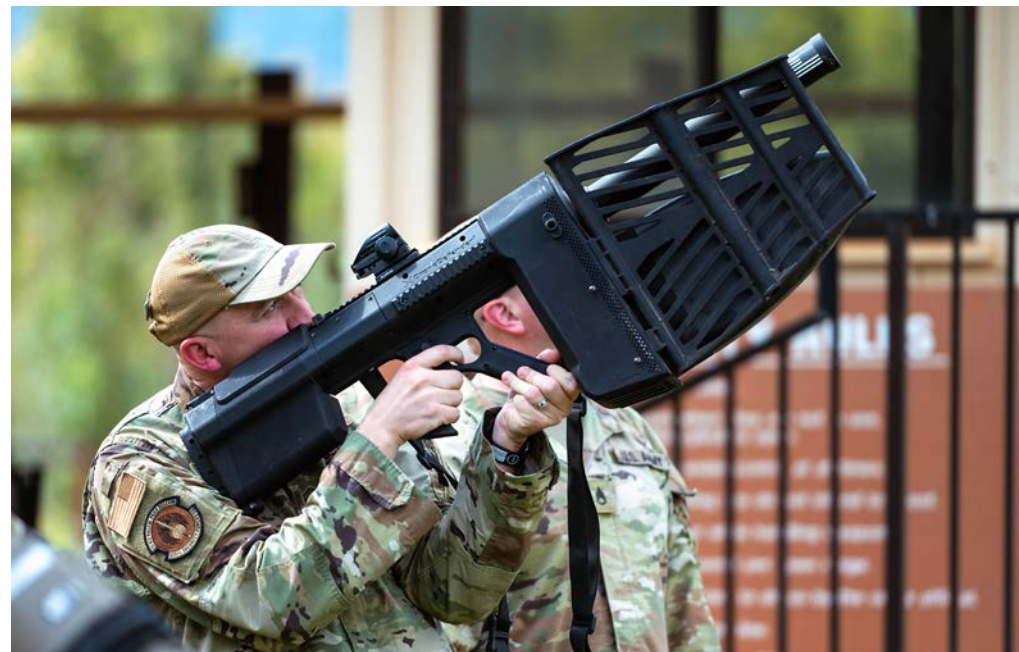
Master Sgt. David Rogers, 315th Security Forces Squadron fire team leader, aims a DroneDefender weapon at a small unmanned aircraft system during Exercise NEXUS FORGE Feb. 5, 2025, at Schofield Barracks, Hawaii. Adversaries continue to refine drone tactics, increasing the need for adaptable training and emerging technologies to maintain airspace dominance. (Air Force photo by Master Sgt. Jeffrey Grossi)
