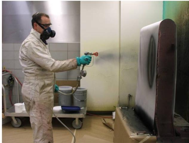
FIGURE A-7. Reaction spray of elastomeric coating.
