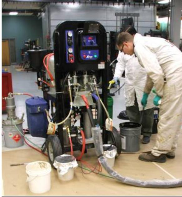
FIGURE A-3. Plural component reaction spray equipment.
